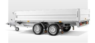
Extended sidewalls increase the height from 300/350 to 500 mm -
