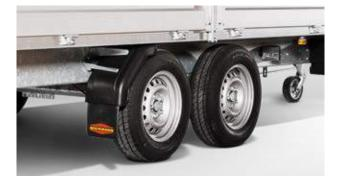
Impact-resistant, recyclable plastic mudguards The standard HL-AL trailers are equipped with an impact-resistant, recyclable plastic mudguard (HL-AL-F series with two mudguards).
