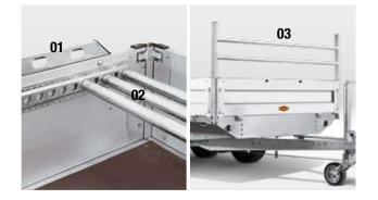
**Transport locking device** Use sidewall gallery (01) and shut-off bars with anchor rail (02) to securely lashing the cargo. The front ladder rack (03) increases transport and driving safety – especially when transporting tall goods.
