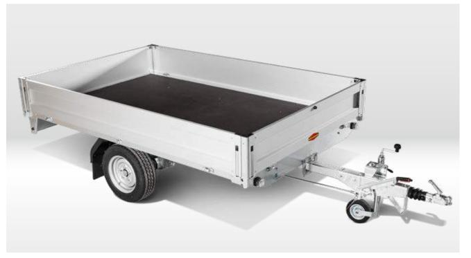
Large loading volume Full utilization of the loading area with 300 mm high aluminium sidewalls.
