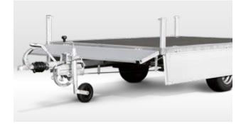
Foldable sidewalls on all 4 sides for comfortable loading and unloading from all sides
