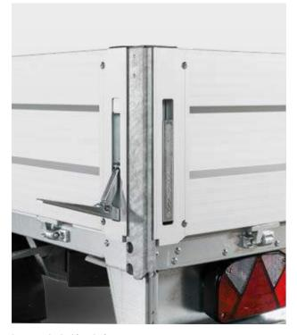
Long-stroke locking device to safely and quickly release and fix the sidewalls.
