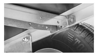
**Crossbeams** Full length, solid steel crossbeams ensure a high torsional rigidity.
