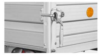
Angle lever lock for easy and quick operation.
