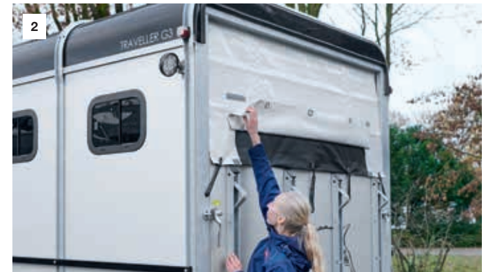
Tarpaulin lift with automatic retraction function [1] and integrated net [2].
