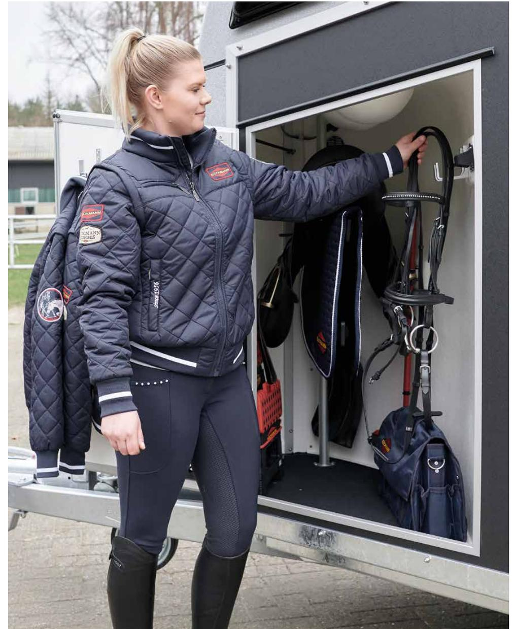
**Duo R tack locker** with storage compartment and extensive standard equipment: pull-out saddle rack, telescopic broom, plastic shovel, door net, mirror, riding crop holder, large bridle hooks and LED light.
